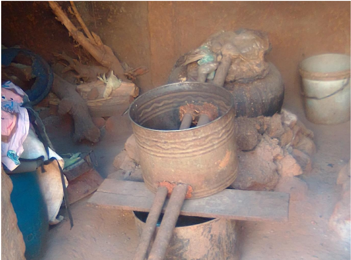
The local distillation apparatus for distilling “Kachasu”
